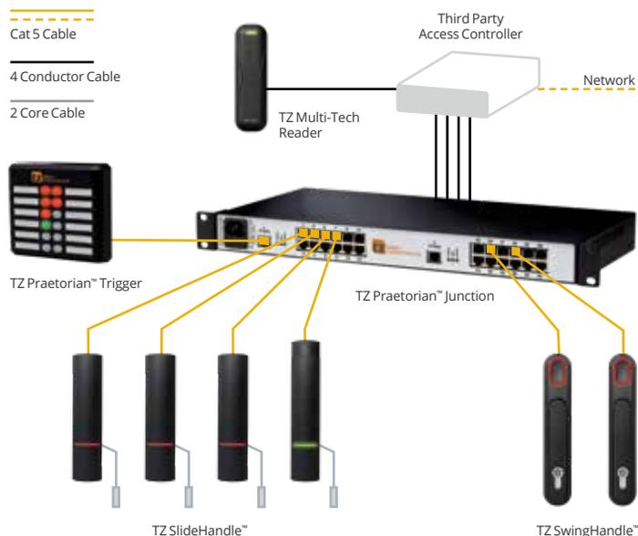
The TZ Praetorian System has been designed for the needs of data centers and IT professionals to bridge the gap between the perimeter security provided by building access control systems and the requirements for more granular levels of physical protection at cabinet level.
